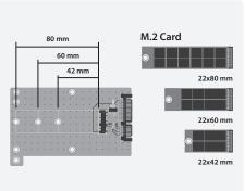
M.2 card comes in different length and 2. sizes (42, 60, 80mm), match your M.2 card length to the hole alignment to decide which mounting hole to use.
