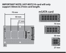
mSATA card comes in different sizes 2. (27, 50, or 70mm), match your mSATA card size to the hole alignment to decide which mounting hole or clip to use.
