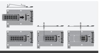
Attached mSATA Device by inserting the mSATA Card and securing the using the latch to lock or using the washer and screw to hold the mSATA card in place.
