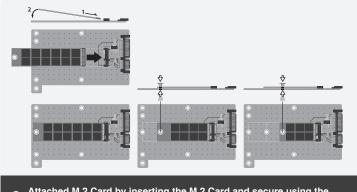
Attached M.2 Card by inserting the M.2 Card and secure using the 2. Attached M.2 Card by Inserting the mile 2. washer and screw to hold the M.2 card in place.
