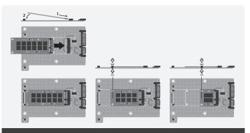
Attached mSATA Device by inserting the mSATA Card and securing the using the latch to lock or using the washer and screw to hold the mSATA card in place.
