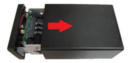
3. Insert the Second (lower) HDD/SSD in to the lower bay and push all the way in for the SATA interface on the tray to make full contact with the drive interface. The screw hole on the drive should align with the tray screw hole.
