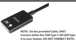
8. Connect the USB cable to the DOCK and your computer. If your computer is powered ON, you should see a red LED on the DOCK (the RED LED indicates the DOCK is getting power from the USB Bus. BUT the DOCK POWER is OFF).
