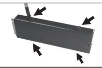
Align the heatsink side hole to the metal casing and fasten the four screws (two on each side) to hold the NVMe module in place.
