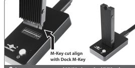
9. Insert your mounted NVMe into the NVMe slot on the DOCK and make sure it is fully inserted. NOTE the M key and align the interface correctly before inserting it.
