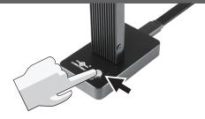
10. Press the power button to turn ON the DOCK and the LED should turn white (the WHITE LED indicates the DOCK is POWERED ON) the NVMe is ready for use.
