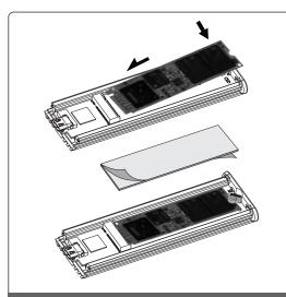
4. Align your NVMe Module to the NVMe interface (Align the notch on your module with the interface notch) Insert your NVMe at an angle all the way in and push the end down to lock NMVe using the PEG in mention is Step 3 to rotate the lever clockwise from position "B" to position "C". Remove both sides of the protective film off the thermal pad and place the Thermal pad on top of your NVMe module.
