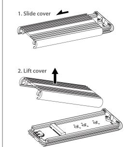
2. Slide the cover in the direction shown and lift the cover. Slide the PCB out of the bottom casing (note the guide rail).
