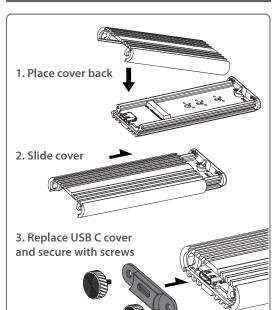
5. Cover back the top cover, the USB C cover plate, and secure using the two thumbscrews. Your Storage is ready for use.
