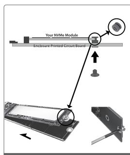
5. Use the screw nut provided, insert into the semi-circular notch of your M.2 module, press down the M.2 module and secure the M.2 screw nut using the screw from the underside.
