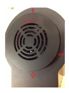
4) Remove the 4 mounting screws and unplug the fan connector. Note the color code.
